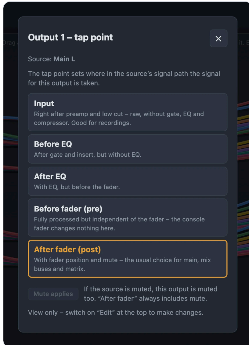
Tapping an output: the tap point with explanation
